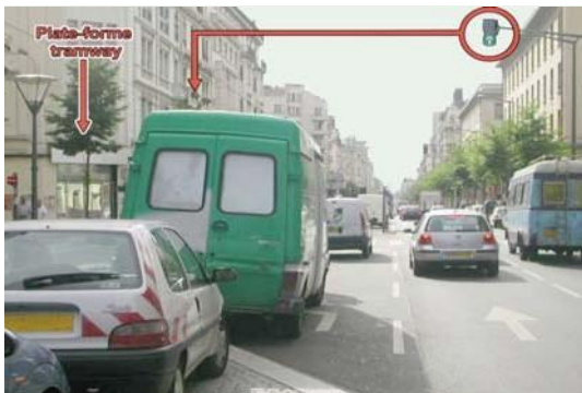
The left-turn directional traffic light (different from the straight-on light on the overhead post) is masked by the van parked on the road lane for a user who has to cross the tram tracks
