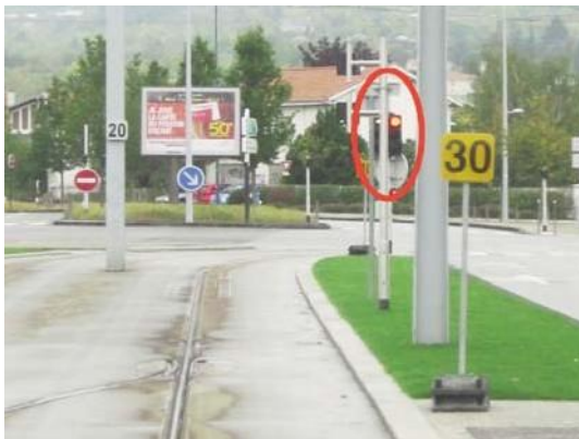
Structure upstream of the R17 signal making it less visible
