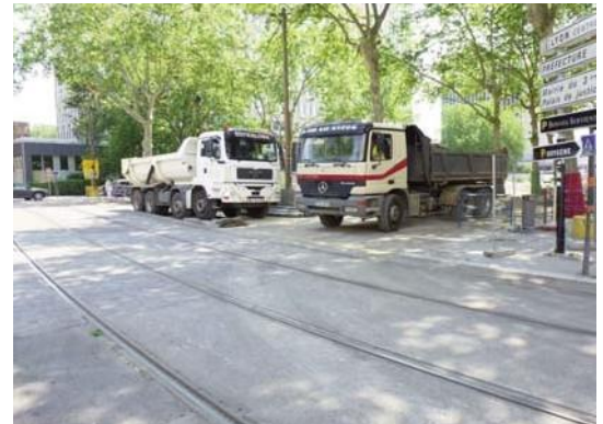
Construction vehicles masking visibility at the approach to an intersection
