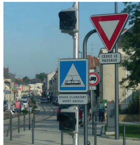
Photo 15: the R24 barrier signals are doubled at different heights to enhance their perception (source STRMTG)
