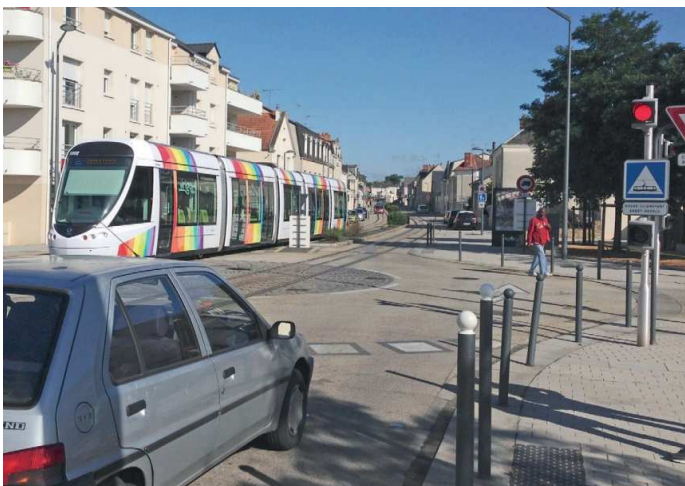
Photo 16: at this mini-roundabout at a general traffic entry section, the traffic lights for vehicles can be installed only at the entries (source STRMTG).
